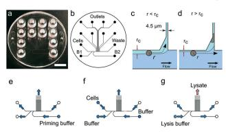
Fig. 1 Device design and operation. (a) Image of the single use polymer device. Scale bar is 1 cm. (b) Microfluidics layout. (c) Conditions for cell trapping an unoccupied trap  $r < r_c$ . (d) The trapped cell reduces the flow through the trap such that for the next incoming cell,  $r > r_c$ . (e-g) Flow directions in the device under priming, cell capture and lysis.
