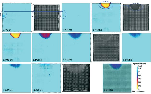
Fig. 2 (a)-(i) Measured time-lapse optical opacity images of on-chip cultured fibroblasts for cell growth assays together with the corresponding reference stereo-microscope images. (j) The reference stereo-microscope image and the CMOS optical opacity image at t = 72 h are superimposed to show on-chip fibroblast location and matching. All optical opacity images use the same scale as that in (j).
