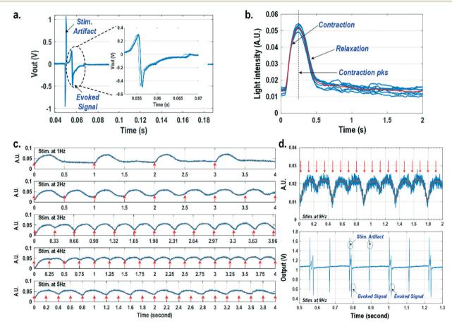
Fig. 6 (a) The overlay plot of the measured extracellular potentials with a current stimulation pulse width of 800 μs. (b) The overlay plot of the measured optical signals at a stimulation rate of 0.5 Hz. (c) The measured optical signals at different stimulation rates. (d) The measured optical signals and extracellular potentials at a stimulation rate of 9 Hz.
