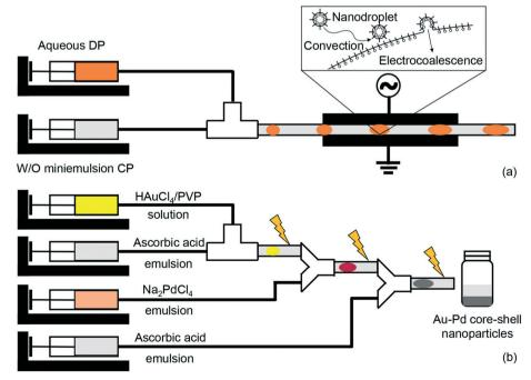
Fig. 1 (a) Experimental setup for generating agueous microdroplets with a W/O miniemulsion and electrocoalescence. (b) Three electrocoalescence-assisted chemical addition steps for Au-Pd core-shell nanoparticle synthesis.
