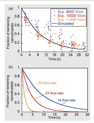
Fig. 7 (a) Simulation of the convection-controlled scenario and comparison to experimental results under a CP flow rate of 50  $\mu L$  min $^{-1}$ and DP flow rate of 10 µL min<sup>-1</sup>. (b) Convection-controlled simulation results at 5×, 2×, and 1× of the base flow rate of 50  $\mu$ L min<sup>-1</sup> (CP) and
