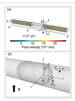
Fig. 6 (a) Convective fluid field of the continuous phase outside the microdroplet. Values represent the velocity of the continuous phase flow. (b) An illustration of the r and  $\theta$ -direction electrostatic forces in a spherical coordinate defined orthogonal to the cylindrical tubing.
