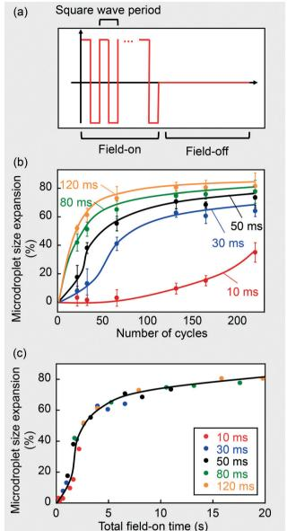
Fig. 3 (a) An illustration of a field on-and-off cycle. (b) Microdroplet size expansion with number of cycles for five different field-on times in each cycle. Solid lines are added manually to emphasize trends (error bars were obtained with three repetitions and corresponded to a 95% confidence interval). (c) Microdroplet size expansion as a function of total field-on time only.
