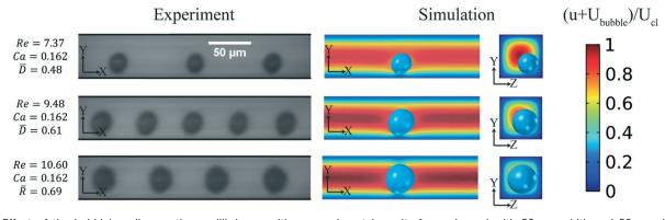
Fig. 8 Effect of the bubble's radius on the equilibrium position: experimental results for a channel with 50 μm width and 50 μm depth are compared with the corresponding simulations in color. The color map shows the normalized velocity of the flow in the x-direction. The results show that the equilibrium position of larger bubbles is closer to the centerline than that of smaller bubbles.
