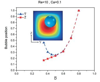
Fig. 9 Numerical simulations of different bubble diameters for the square channel at constant Re = 10 and Ca = 0.1. The initial position of the bubble is at  $(\bar{Y}, \bar{Z}) = (0.7667, 0.6)$ . The equilibrium position of a bubble that is smaller than half of the channel width is close to the wall. A bubble larger than half of the channel width moves along the diagonal of the channel and by increasing the diameter of the bubble. it eventually moves to the center of the channel.
