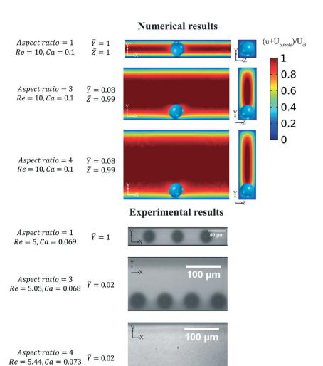
Fig. 10 Effect of the channel geometry on the lateral position of the bubble while the Re and Ca are constant. Experimental and numerical results show that in the wider channels, the bubble equilibrium position is close to the smaller edge while in the channel with an aspect ratio of one the bubble equilibrium position is in the center.
