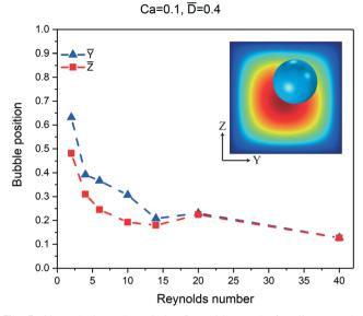
Fig. 5 Numerical results of the Reynolds number's effect on the lateral position of a bubble in a square channel. The blue points and the red points show the equilibrium position of the bubble in the horizontal and vertical directions, respectively. All simulations are carried out for  $\bar{D}$  = 0.4 and Ca = 0.1. The initial bubble position is at  $(\bar{Y}, \bar{Y})$  $\bar{Z}$ ) = (0.7667, 0.6).
