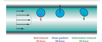
Fig. 1 Forces acting on the bubble: a wall-induced lift directing towards the centerline which diminishes as the bubble moves away from the wall, a shear gradient lift that pushes the bubble towards the wall. and a deformation-induced lift pointing towards the centerline which becomes stronger as the bubble deformation increases.
