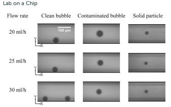
Fig. 12 Experimental results show different equilibrium position for bubbles and particles: addition of a small amount of surfactant forces the bubble to behave like a particle. At the same flow rate, the equilibrium positions of contaminated bubbles and solid particles are at the center of the wider channel while clean bubbles stay close to the shallower wall.
