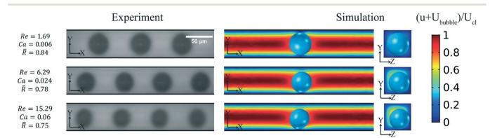
Fig. 4 Effect of Re on the lateral position of the bubble: experimental results and the corresponding numerical simulations are for the channel with 50 µm width and 50 µm depth. The bubble diameter is normalized to the channel width. By increasing the Re, the bubble moves gradually towards the wall
