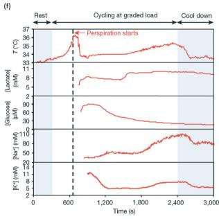
Fig. 17 Bringing electrochemical sensors directly onto skin to detect sweat (adapted). 158 In all the examples provided in the figure, technology is mechanically compliant to skin, which is a first step to reduce the sweat volume between skin and sensors. The data shown in (f) is for a human subject wearing the technology shown in (d). 178
