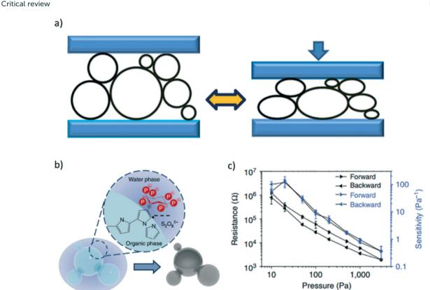
Fig. 8 a) Schematic illustration of the elasticity of hollow sphere structured polypyrrole (PPy). b) Schematic illustration of the phase separation between water and organic components for the synthesis of PPy hydrogels. c) Electrical resistance response to induced pressure.<sup>84</sup>
