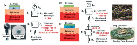
Fig. 3 Equivalent circuit models of electrode-skin interfaces for different electrode designs. (a) Gel electrodes, including wet and solid forms (disposable deep EEG cup electrode, Rhythmlink; ECG electrode H1354LG, Kendall). (b) Dry contact electrodes. 61 (c) Dry capacitive (non-contact) electrodes.51
