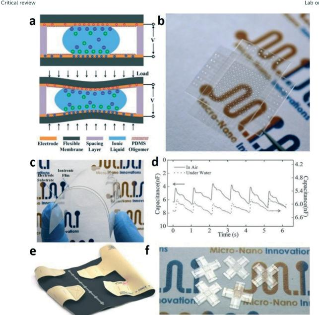
Fig. 10 (a) Iontronic droplet sensor operation principle. (b) Photo of an iontronic microdroplet sensing array. (c) Photo of a flexible ionic gel film on an electrode substrate. (d) Real-time pulse pressure waveforms in dry and underwater environments. (e) Photo of a commercial inelastic legging integrated with the iontronic flexible sensing array. (f) Prototypes of microfluidic tactile sensors for three-dimensional force measurements.
