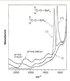
**Fig. 5** IR spectra of (i) HF-SbF<sub>5</sub>, (ii) HF-SbF<sub>5</sub> +  $^{12}$ CO, and (iii) HF-SbF<sub>5</sub> +  $^{13}$ CO. Modified with permission from ref. 166. Copyright of The American Association for the Advancement of Science (1997).
