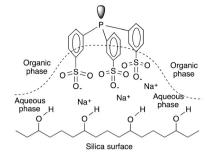
Fig. 4 Schematic representation of the immobilization of TPPTS on silica. Modified with permission from ref. 149. Copyright of Springer (1990).
