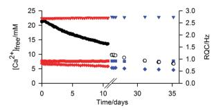
Fig. 6 Plots of  $[Ca^{2+}]_{free}$  in  $2/CaCl_2$  gel versus time after an NaCl solution was placed on top of the sample. After the first solution (black circle) had stood on top of the gel for 26 days, the supernatant solution was removed, fresh solution placed on top and the second series of measurements (white) commenced. The RQCs of HDO (square), dioxane (down triangle) and formate (diamond) are plotted for the first (red) and second (blue) series of measurements.
