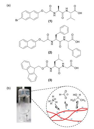
Fig. 1 (a) Structure of the gelators used in this work. (b) Cartoon to illustrate the general concept of this work: self-supporting hydrogels can be prepared from a variety of gelators and by a variety of methods. By studying the relative affinities of a set of probe molecules and ions for the surface of the gel fibres (red) we are able to measure the surface chemical properties
