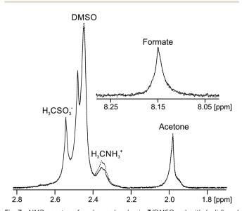
Fig. 7 NMR spectra of probe molecules in 3/DMSO gel with (solid) and without (dashed) on resonance pre-saturation applied to the gel fibres. The downfield and upfield resonances of acetone and DMSO correspond to the totally protonated (H<sub>6</sub>) and partially deuterated (HD<sub>5</sub>) molecules respectively. The formate resonance is shown inset.
