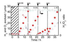
Fig. 7 Time courses of evolution of H2 and O2 from water over  $Au(1.0)/TiO_2 - NiO_x(0.5)$  under irradiation of visible light from a Xe lamp with various filters. After 13, 21 and 29 h of irradiation and evacuation, the suspension was irradiated again.
