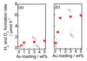
Fig. 6 Effect of Au loading amounts (X) on the rate of evolution of  $H_2$  and  $O_2$  from water over (a)  $Au(X)/TiO_2$  and (b)  $Au(X)/TiO_2-NiO_X(0.5)$  samples under irradiation of visible light.
