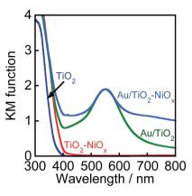
Fig. 2 Absorption spectra of  $TiO_2$ ,  $TiO_2 - NiO_x(0.5)$ ,  $Au(1.0)/TiO_2$ , and  $Au(1.0)/TiO_2 - NiO_x(0.5)$ .
