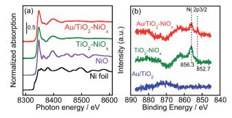
Fig. 4 (a) Ni K-edge XANES spectra of Ni foil, NiO,  $TiO_2-NiO_x(0.5)$  and  $Au(1.0)/TiO_2-NiO_x(0.5)$ ; (b) XPS spectra of  $Au(1.0)/TiO_2$ ,  $TiO_2-NiO_x(0.5)$  and  $Au(1.0)/TiO_2-NiO_x(0.5)$  around Ni 2p components.
