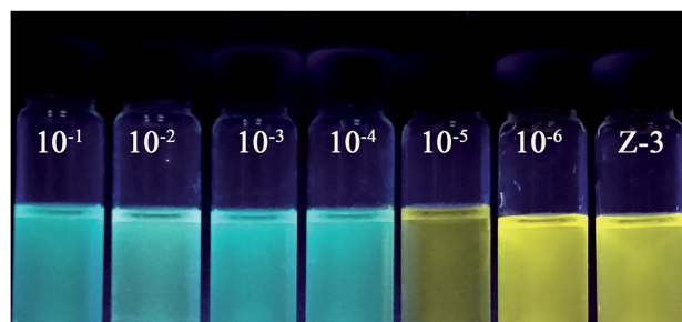
Fig. 6 Naked-eyes detection limit under UV lamp at 365 nm. From left to right, the concentration of Hg 2+ is 10^{-1} \text{ M} , 10^{-2} \text{ M} , 10^{-3} \text{ M} , 10^{-4} \text{ M} , 10^{-5} \text{ M} , 10^{-6} and 0 M.
