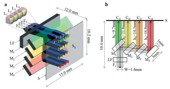
Fig. 2 Design of the developed ultra-small system with a size of 15.0 × 10.2 × 12.0 mm. (a) Perspective view overlaying ray-trace simulation fluxes of rays emitted from  $E_i$  (black lines are rays from  $E_1$  and  $E_3$ , and blue lines are rays from  $E_2$  and  $E_4$ ); LF: long-pass filter;  $S_{ij}$ : image of  $C_{ij}$ . (b) Crosssectional view overlaying complete parallel light fluxes;  $h_i$ : sensor distances for color number j; W: aperture of the system.
