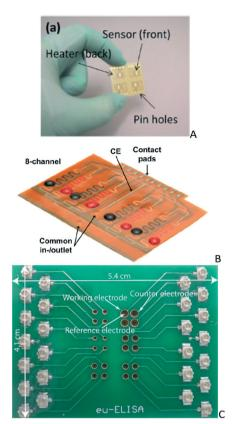
Fig. 9 A) PCB integrating electrochemical sensors and microheaters (reprinted from ref. 133, copyright 2014, with permission from Elsevier), B) photographs of the antibiotic detection microfluidic biosensors comprising eight immobilization sections (reprinted from ref. 136, http://pubs.acs.org/doi/full/10.1021/acs.analchem.6b02294) and C) commercially fabricated microchambers used for IFN- $\gamma$  detection (reprinted from ref. 137, copyright 2016, with permission from Elsevier).
