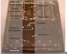
Fig. 6 A) Image of the low-sensing elements and SU-8 microchannel integrated into the PCB (reprinted from ref. 86, copyright 2009, with permission from Elsevier) and B) image of the lab-on-PCB platform for autonomous micromixing (reprinted from ref. 9, copyright 2015, with permission from Elsevier).
