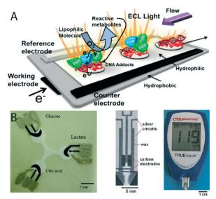
4 A) Paper-based electrochemiluminescence DNA sensors (reprinted with permission from ref. 61, copyright 2013, American Chemical Society) and B) enzymatic ePAD devices (reprinted with permission from ref. 60, copyright 2009, American Chemical Society). 62
