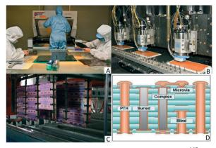
Fig. 11 A) Photopatterning of the resist, courtesy of EPEC; 145 B) CNC drills, courtesy of EPEC;<sup>145</sup> C) industrial wet processing line (© Swoolverton/Wikimedia Commons/CC-BY-SA-3.0, ref. 147); D) schematic of the different via configurations (courtesy of EPP Europe<sup>148</sup>).
