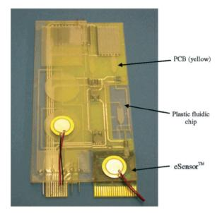
Fig. 7 Self-contained LOPCB integrating reagent storage, valves, pumps, microheaters, PCR chambers and DNA microarray sensors for pathogenic bacteria detection from whole blood (reprinted with permission from ref. 106, copyright 2004, American Chemical Society).
