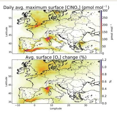
Fig. 11 Mean daily maximum surface ClNO<sub>2</sub> mixing ratios (top) and impact of ClNO<sub>2</sub> production on  $O_3$  (bottom). Inclusion of ClNO<sub>2</sub> leads to small increases in the  $O_3$  mixing ratio predominantly over coastal regions with heavy ship traffic.
