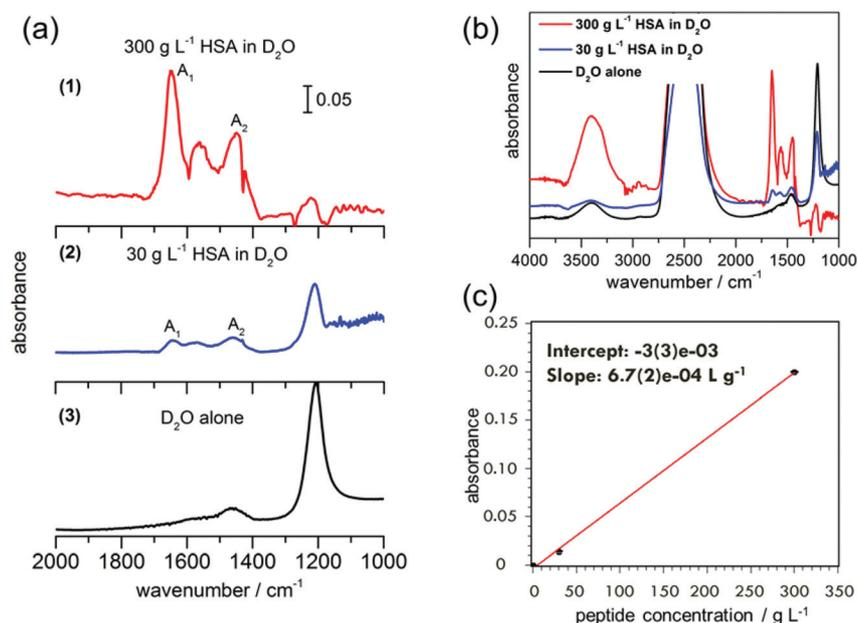
**Fig. 4** (a) ATR-IR spectra of (1) HSA in D<sub>2</sub>O (300 g L<sup>-1</sup>), (2) HSA in D<sub>2</sub>O (30 g L<sup>-1</sup>) in 10 nm deep Ge ATR-IR nanochannel devices and (3) bulk D<sub>2</sub>O alone obtained on the Ge ATR-IR crystal. A1 (1649 cm<sup>-1</sup>) and A2 (1450 cm<sup>-1</sup>) indicate the amide I and amide II peaks, respectively. (b) The extended spectra of the same, from 4000 to 1000 cm<sup>-1</sup>. (c) Peak absorbance of amide I mode versus concentration.
