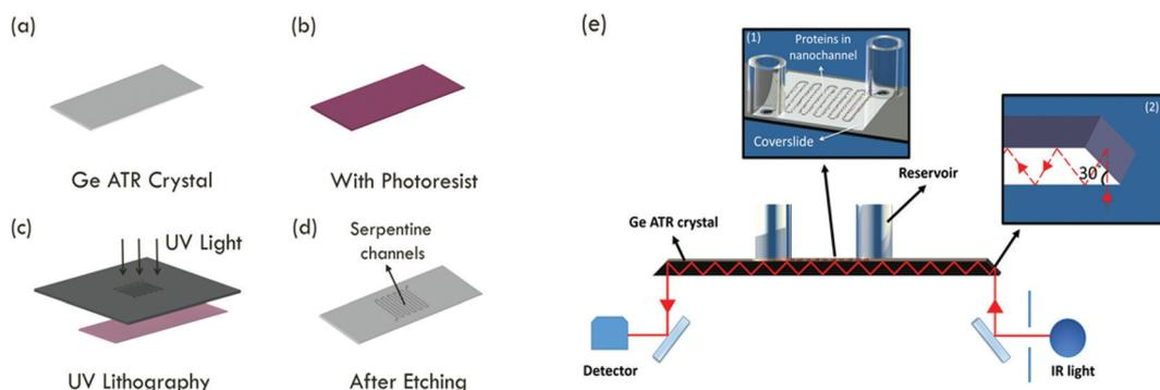
**Fig. 1** (a)–(d) Fabrication scheme of serpentine nanochannels on Ge ATR crystals. (e) Schematic set up for ATR-IR spectroscopy on a Ge nanochannel device. Inset (1) shows an enlarged image of the nanochannel region. Inset (2) shows chip edges ground to 30° angle to facilitate 60° angle of incidence.
