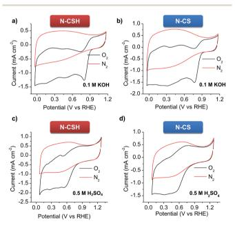
Fig. 3 Cyclic voltammograms of the N-doped carbon microspheres in  $N_2$ - and  $O_2$ -saturated electrolytes at a scan rate of 50 mV s<sup>-1</sup>. (a and b) 0.1 M KOH, and (c and d) 0.5 M H<sub>2</sub>SO<sub>4</sub>.
