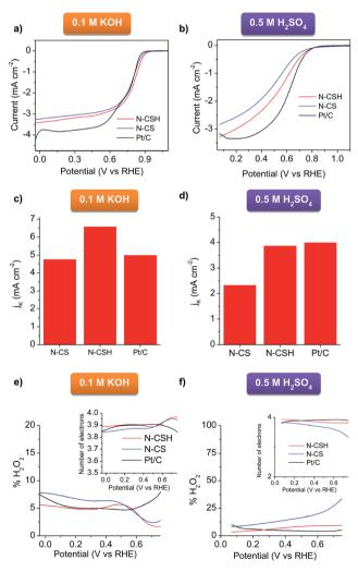
Fig. 4 RDE polarization curves at 1600 rpm for the N-CSH and N-CS samples compared to 20 wt% Pt/C in (a) 0.1 M KOH and (b) 0.5 M H<sub>2</sub>SO<sub>4</sub>, (c) electrochemical activity given as the kinetic-limiting current density  $(J_K)$  at 0.67 V in 0.1 M KOH and (d) at 0.48 V in 0.5 M  $H_2SO_4$ , and peroxide yields of the carbon microspheres in (e) 0.1 M KOH and (f) 0.5 M H<sub>2</sub>SO<sub>4</sub> (inset: variation of the number of electrons with potential).
