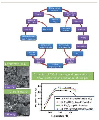
Fig. 9 Preparation flow diagram of low-cost  $deNO_x$  catalyst from blast furnace slag and denitration results. Adapted from ref. 11. Copyright 2014, with permission from Elsevier.
