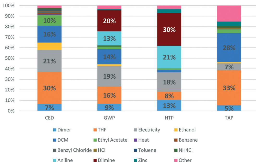
**Fig. 4** Detailed contributions to Recipe impacts of the synthesis of [Pd(IPr\*)(cin)Cl] catalyst.
