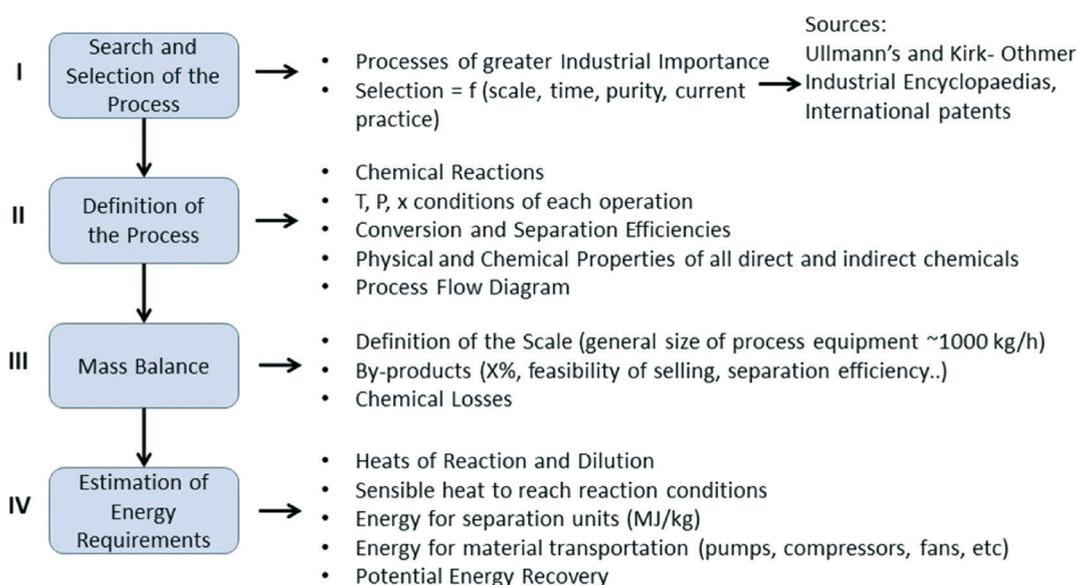
Fig. 1 Development of LCIs for pharmaceutical API manufacture.
