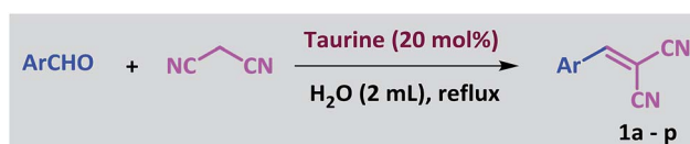
Scheme 1 The Knoevenagel reaction between aldehydes and malononitrile.
