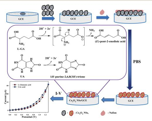
Scheme 3 Fabrication and proposed mechanism for the detection of L-GA and UA by the Co<sub>3</sub>O<sub>4</sub> NSs
