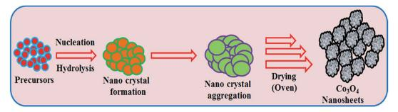
Scheme 2 Growth mechanism of mesoporous Co<sub>3</sub>O<sub>4</sub> nanosheets
