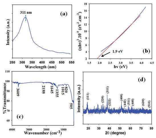
Fig. 1 (a) UV spectrum, (b) band-gap energy plot, (c) FTIR and (d) XRD pattern of the NSs
