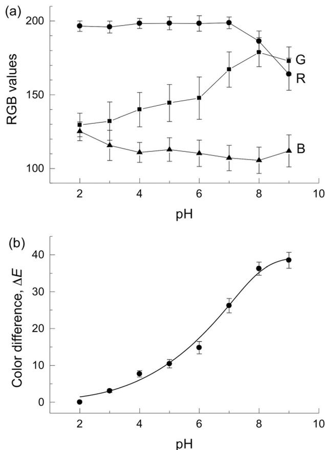
Fig. 2 Plots of (a) R, G, and B against pH value and (b) plot of CIE  $L^*a^*b^*$  color difference against pH value. Data points represent the mean of 3 measurements and error bars represent one standard deviation from the mean. In panel (b), data were fitted to a sigmoidal curve ( $R^2 = 0.982$ ).
