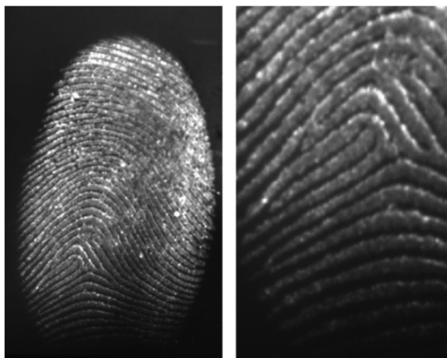
Fig. 11 A charged latent fingerprint on a PVDF substrate developed by using the aptamer-based reagent. The fingerprint was aged for 24 hours before it was developed with the lysozyme aptamer 1 reagent containing CAL Fluor® Orange 560 as the fluorescent tag. 91 Reproduced from ref. 91 with permission from Wiley.
