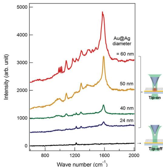
**Fig. 4** A set of BPT TERS spectra with (tip-on, colored lines) and without (tip-off, black line) Au@Ag NP-tips. The same BPT sample was used for all of the measurements. Each spectrum was obtained with a laser power of 20  $\mu\text{W}$ , and the integration time was 180 s. For the ease of viewing, each of the spectra is vertically offset.
