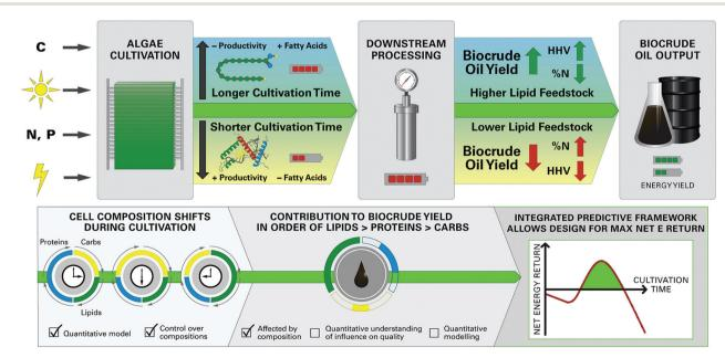
Fig. 1 The integrated modeling framework allows for prediction and optimization of system-scale parameters for the microalgae-HTL biofuel system. The top half of the figure represents the integrated processing scheme for microalgae HTL, with the black arrows representing decisions on cultivation times that lead to downstream implications. The bottom half represents the current research progress towards formulating an integrated predictive framework
