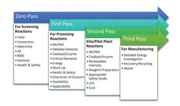
Fig. 2 Structure of the metrics toolkit showing the parameters covered at each Pass.
