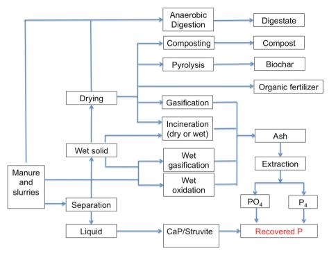
Fig. 4 Schematic overview of the main options to recover P from manures and biosolids. Adapted from Oenema et al.<sup>53</sup> and Schoumans et al.<sup>55</sup>
