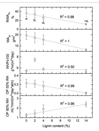
Fig. 10 Relative water absorption of the nanopapers after 2 h of immersion in water ( $RWA_{2h}$ ), water absorption ( $WA_{2h}$ ) and barrier properties (WVP and OP) of the nanopapers evaluated as a function of the lignin content.
