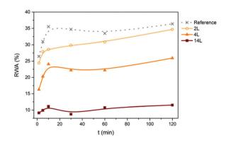
Fig. 9 Relative water absorption (RWA) of the nanopapers with different lignin content measured after different immersion times in water.
