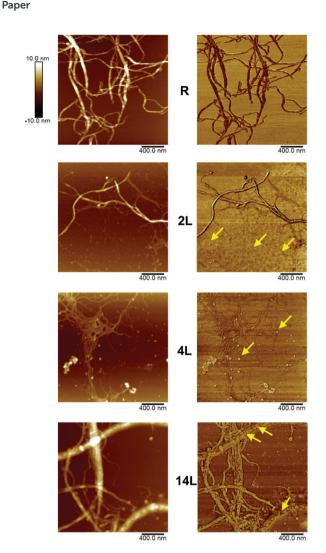
Fig. 3 AFM images of 4  $\mu m^2$  areas of LCNF (samples 2L, 4L and 14L) as well as the reference CNF (R), deposited on mica after air-drying from diluted aqueous suspensions. The height and phase images are presented in the left and right columns, respectively. The arrows point to some of the lignin nanoparticles, which act as a cementing material between the cellulose nanofibrils.
