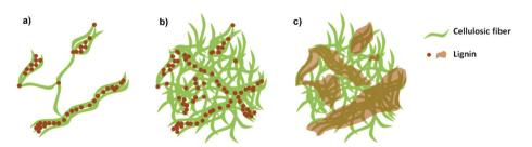
Fig. 5 Proposed model to describe the location of the lignin within nanofibril suspensions and nanopapers. (a) LCNF suspension, (b) LCNF suspension, sion after filtering, (c) LCNF nanopaper after pressing.
