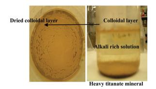
Fig. 15 The photograph of the leaching mixture (right) which was allowed to settle after roasting of ilmenite. The leaching was carried out with the deionized water at room temperature for 30 minutes. The dried colloidal product (left) on filter paper is shown.<sup>68</sup>
