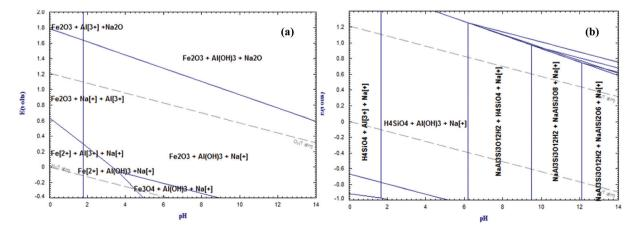
Fig. 11 (a)  $E_h$ -pH diagram of the system Na-Al-Fe-H<sub>2</sub>O at 50 °C and 1 atm. (b)  $E_h$ -pH diagram of the system Na-Al-Si-H<sub>2</sub>O at 50 °C and 1 atm. <sup>66</sup>
