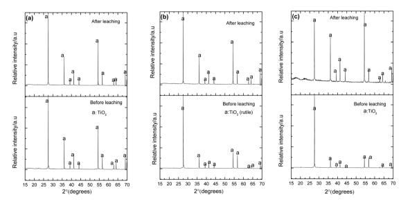
Fig. 24 XRD patterns of sintered pellets with 1.3 (a), 4.3 (b) and 8.6 (c) mol%  $V_2O_5$  before and after leaching. The diffraction data compare well with the ICDD references: 04-008-7811 (TiO<sub>2</sub>).
