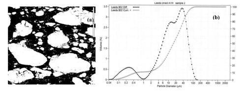
Fig. 12 (a) Scanning electron micrograph of the alumina extracted (100 µm). (b) Cumulative distribution values with bimodal particle size distribution of calcined alumina.
