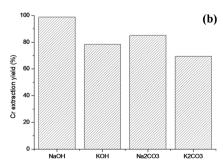
Fig. 17 (a) Chromium extraction yields after roasting at 1000 °C for 2 hours in air and water leaching at 50 °C for 45 minutes with different alkali salts. (b) Chromium extraction yields after roasting at 1000 °C for 2 hours and water leaching at 50 °C for 45 minutes with different alkali salts under a richer oxygen atmosphere with intermittent stirring.
