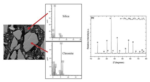
Fig. 7 (a) Back-scattered scanning electron image of the chromite concentrate showing the different mineral constituents (100  $\mu$ m). (b) The X-ray powder diffraction data of the as received South African chromite concentrate compare well with the ICDD reference: 01-070-6389(Fe<sub>0.51</sub>Mg<sub>0.49</sub>)-(Cr<sub>0.73</sub>Al<sub>0.27</sub>)<sub>2</sub>O<sub>4</sub>.
