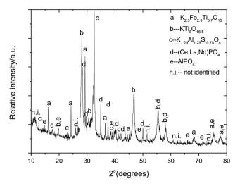
Fig. 14 X-ray powder diffraction pattern of the reaction product formed as a result of chemical reaction between K2CO3 and FeTiO3 at 825 °C for 4 hours in air. The main phases compare well with the ICDD references: 00-041-1100 K<sub>2</sub>O·8TiO<sub>2</sub>00-040-0960 K<sub>2.3</sub>Fe<sub>2.3</sub>Ti<sub>5.7</sub>O<sub>16</sub>, 00-032-0731  $K_{1.25}Al_{1.25}Si_{0.75}O_4$ , 00-046-1295 (Ce, La, Nd)PO<sub>4</sub> and 04-009-5769 Al(PO<sub>4</sub>).
