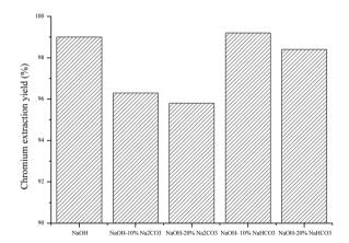
Fig. 20 Chromium extraction yields after roasting at 1000 °C for 2 hours under a 30%  $O_2$ –70%  $N_2$  atmosphere with intermittent stirring and water leaching at 50 °C for 45 minutes with different sodium salts.
