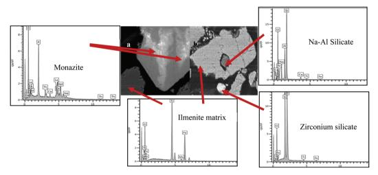
Fig. 5 Back-scattered scanning electron image of Bomar ilmenite showing the different mineral constituents: (a) non-magnetic fraction (50 µm) (b) magnetic fraction (50 µm).
