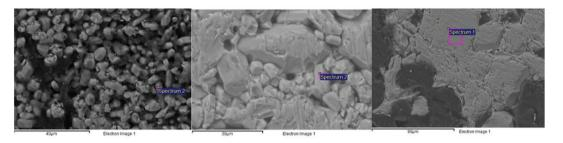
Fig. 23 SEM images for the  $TiO_2-V_2O_5$  mixtures after sintering at 1100 °C for 24 hours, 1.3 mol%  $V_2O_5$  (left), 4.3 mol%  $V_2O_5$  (middle), 8.6 mol%  $V_2O_5$  (right).
