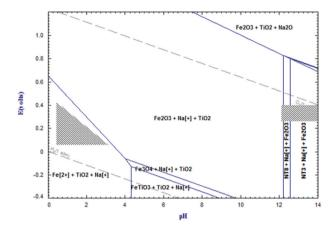
Fig. 16 The  $E_h$ -pH diagram of the system Na-Ti-Fe-O calculated by Fact-Sage 6.4 software at 70 °C. NT3: Na<sub>2</sub>TiO<sub>3</sub>, NT8: Na<sub>8</sub>Ti<sub>5</sub>O<sub>14</sub>.66
