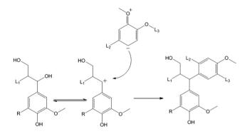
Fig. 8 Condensation of the lignin via benzylic carbonium ion formation after heterolytic cleavage of the benzylic C-O bonds [L<sub>1</sub>, L<sub>2</sub>, L<sub>3</sub> = lignin fragments; R = H or OMe].
