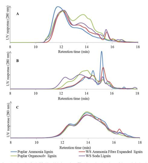
Fig. 2 GPC profiles of acetylated starting lignin (A), thioacidolysis products (B) and acetylated products of the catalytic depolymerisation at 300 °C and 20 bar H<sub>2</sub> (C).
