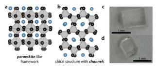
Fig. 1 Schematics of the two structure types observed in the series  $[NH_3NH_2]B(HCOO)_3$  with B = Mn<sup>2+</sup>, Co<sup>2+</sup>, Zn<sup>2+</sup> and Mg<sup>2+</sup>. The structures are simplified to emphasize the perovskite-structure motif in (a) and the hexagonal channels in (b). Grey polyhedrons are ZnO<sub>6</sub> octahedrons, black spheres formate anions and blue spheres correspond to [NH3NH2]+ cations. (c and d) Show crystals of Zn-1 (c) and Zn-2 (d), see ESI† for more crystals.
