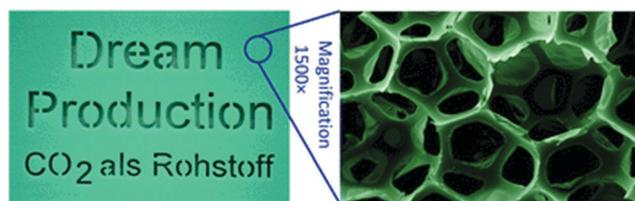
Fig. 17 Shows an image of a polyurethane foam and micrograph showing the foam structure. The foam was prepared by the reaction between poly(ether carbonate) polyol (10.5 wt% CO<sub>2</sub>) and toluene di-isocyanate. The images are reproduced from ref. 4.
