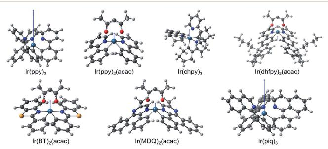
Fig. 3 DFT optimized molecular structure, calculated relative magnitude and orientation of permanent dipole moment  $\mu$  (blue arrows) for all phosphorescent emitter molecules investigated here. All dipole moments originate at the center of charge.
