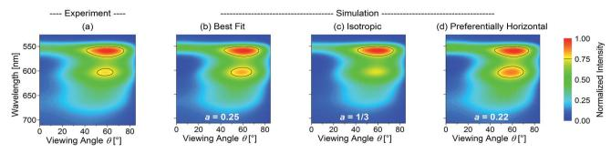
Fig. 2 TM-polarized part of the spectral radiant intensity for the OLED stack with  $Ir(dhfpy)_2(acac)$ . (a) Experimental data, (b) simulated data for the best fit (a = 0.25), (c) simulation assuming isotropic orientation (a = 1/3) and (d) simulation assuming slightly stronger horizontal orientation (a = 0.22). All intensities are normalized to the maximum intensity and are plotted on a linear false-color scale.
