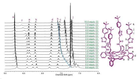
Fig. 3 Partial <sup>1</sup>H NMR spectra of receptor 6 upon addition of equivalents of TBA·CI (500 MHz, 293 K, CDCl<sub>3</sub>).
