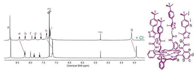
Fig. 2 Partial <sup>1</sup>H NMR spectra of (a) receptor 5 and (b) receptor 5 and one equivalent of TBA·Cl (500 MHz, CDCl<sub>3</sub>, 293 K).
