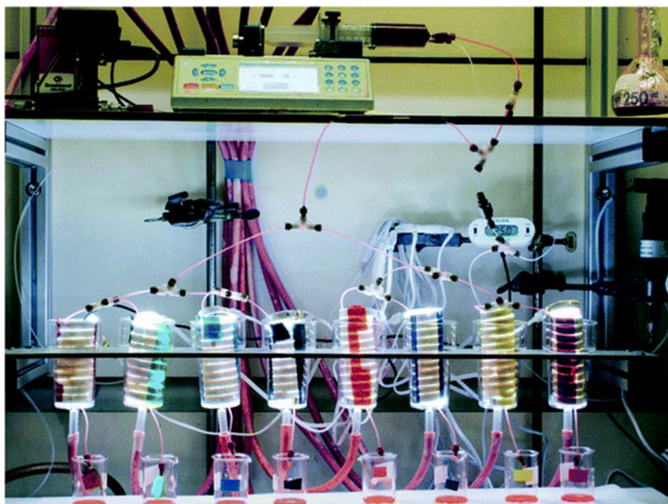
Fig. 16 (a) Schematic overview of the 8-capillary microreactor system, (b) a picture of the 8-capillary microreactor system with a gas–liquid photocatalytic transformation running. Reproduced from ref. 250 with permission from Chemistry Europe.
