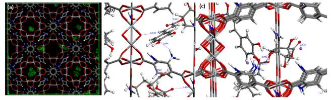
(a) Density of presence for the CGA (green dots) in MIL-125-NH<sub>2</sub> obtained from GCMC simulations, (b) snapshots illustrating the main interactions between the neutral CGA and the MOF, and (c) snapshots illustrating the main interactions between the ionic CGA (compensated by Na<sup>+</sup>) and the MOF. The colours of the atoms are the following: H (white), C (black), O (red), N(blue) and Ti (grey).
