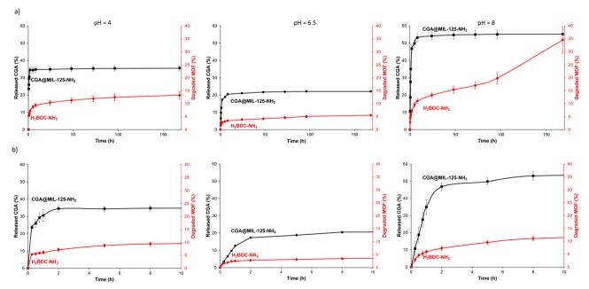
Fig. 3 CGA release (black squares) from CGA@MIL-125-NH2 and leached linker (H2BDC-NH2, red circles) in aqueous media at different pHs (4, 6.5, and 8 from left to right) during (a) 168 h (7 days), and (b) 10 h.
