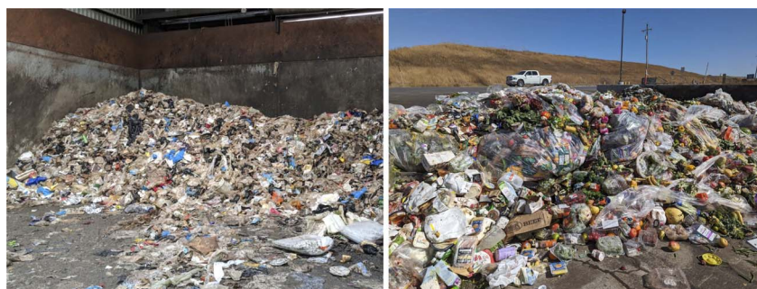
Fig. 3 Images of plastic contamination in organic waste streams. Photos taken at Zero Waste Energy Development Company in San Jose, CA and Yolo County Central Landfill in Woodland, CA. Photo credit (both): Corinne Scown.
