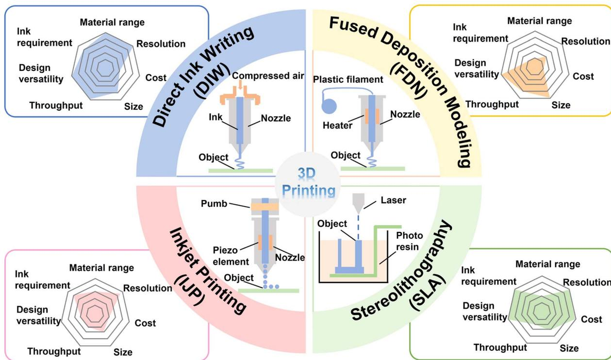
Fig. 2 Schematic of printing and characteristics of four representative 3D printing techniques (DIW, FDM, IJP and SLA) to fabricate MBs.
