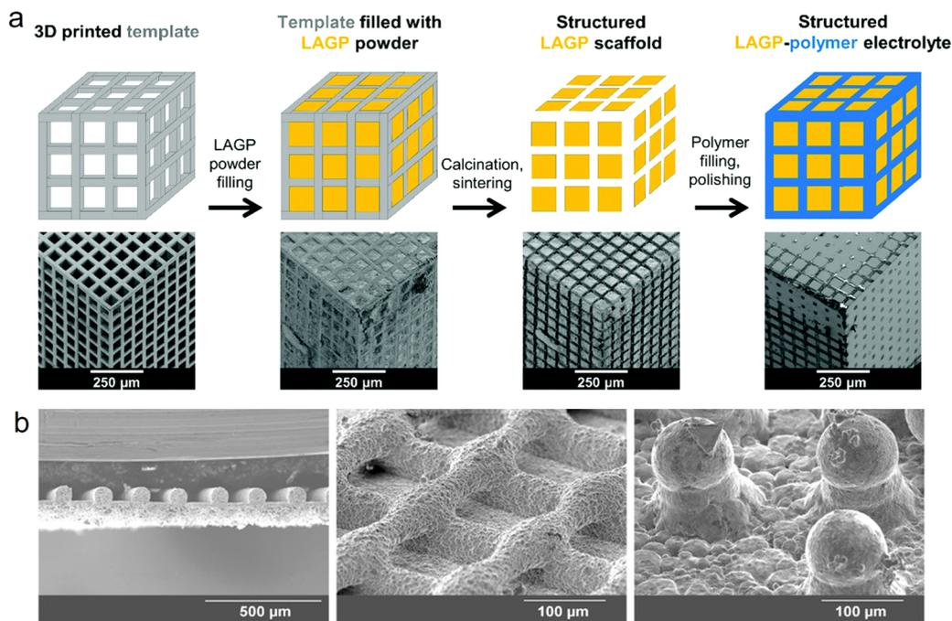
Fig. 9 3D-printed ceramic-based solid-state electrolytes. (a) Schematic illustration of the preparation process of 3D-printed LAGP electrolytes. Reproduced from ref. 203. Copyright 2018, The Royal Society of Chemistry. (b) SEM images of 3D-printed LLZO electrolytes at different magnifications. Reproduced from ref. 202. Copyright 2018, Wiley-VCH.
