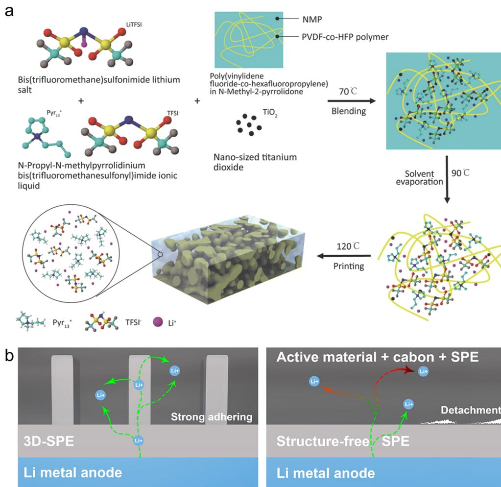
**Fig. 8** 3D-printed hybrid-based solid-state electrolytes. (a) Schematic illustration of the composition and preparation process of 3D-printed Pyr<sub>13</sub>TFSI-based electrolyte inks. Reproduced from ref. 199 Copyright 2018, Wiley-VCH. (b) Schematic of 3D-printed and structure-free electrolytes via SLP method (SPE: solid polymer electrolyte). Reproduced from ref. 200. Copyright 2020, The American Chemical Society.
