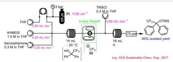
Scheme 12 Reaction monitoring using FlowIR of the use of trifluoromethane 31 to generated functionalised fluorinated compounds in a telescoped flow process.53
