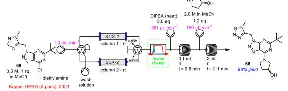
Scheme 25 Telescoped amine scavenging with nucleophilic aromatic substitution in flow using in-line UV-vis spectrometry developed by Kappe and co-workers. 67,68
