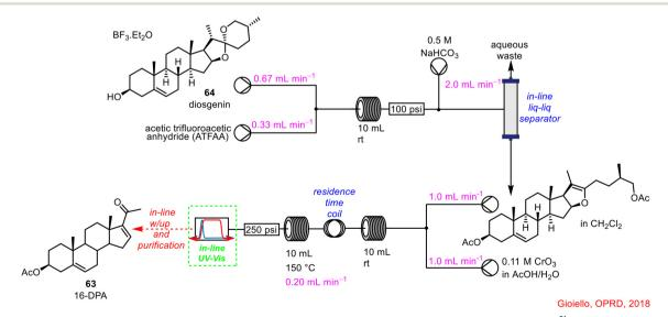
Scheme 23 Telescoped flow synthesis of 16-DPA using in-line UV-vis spectroscopy to monitor reaction completion. 61
