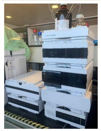
Fig. 4 Typical HPLC set-up that can be adapted for use in continuous flow processes.
