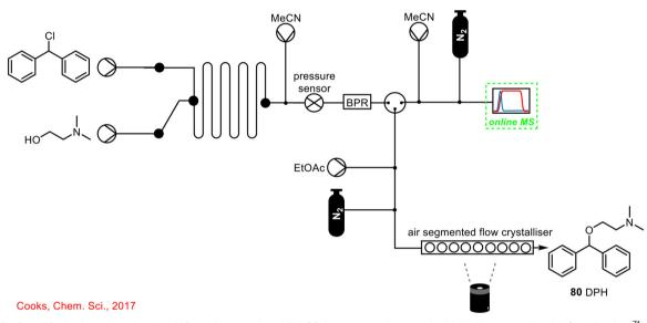
Scheme 30 Simplified schematic of online MS used to monitor DPH 80 formation telescoped with in-line crystallisation/purification.<sup>71</sup>
