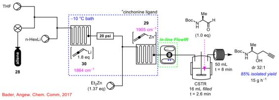
Scheme 11 Use of in-line FlowIR in the telescoped synthesis of homopropargyl  $\beta$ -amino alcohols. 50
