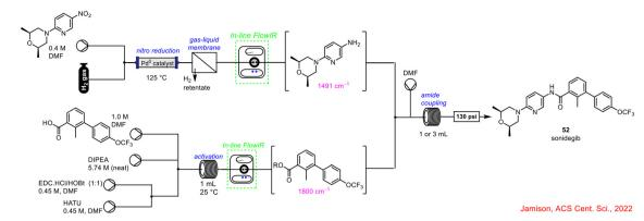
Scheme 19 Schematic of flow synthesis of sonidegib 52 (ref. 58).
