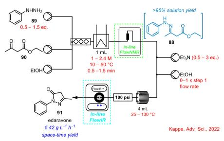
Scheme 35 Telescoped two-step synthesis of API edavarone using in-line FlowNMR to monitor initial imine formation step. 76
