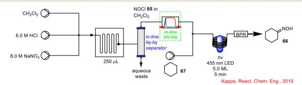
Scheme 24 Telescoped NOCI 65 generation with photochemical synthesis of cyclohexanone oxime 66 using in-line UV-vis spectrometry to monitor NOCl 65 concentration.64
