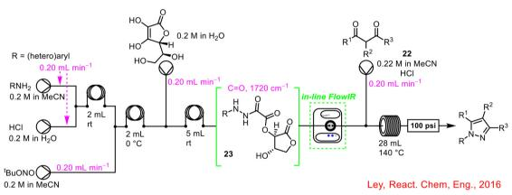
Scheme 9 In-line FlowIR used to develop the four-step telescoped continuous synthesis of pyrazoles. 48
