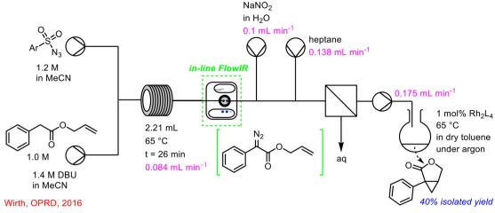
Scheme 8 Use of in-line FlowIR to monitor diazo transfer reaction in telescoped synthesis of lactones.<sup>47</sup>
