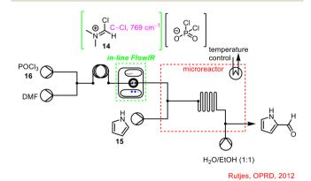
Scheme 5 In-line FlowIR flow cell used to monitor conversion of POCl<sub>3</sub> **16** in the telescoped process to synthesise 2-formylpyrrole **17** (ref. 43).
