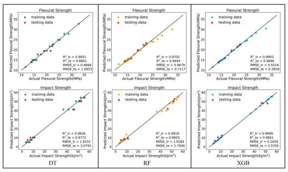
Fig. 2 Parity plots of DT, RF, and XGB models using structural characteristics to predict mechanical properties; the reference line (y = x)represents perfect prediction alignment between actual and predicted values.
