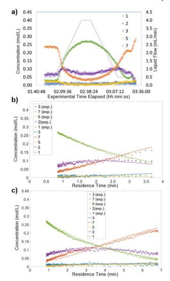
Fig. 4 Reaction concentration analysis for Pt/Al<sub>2</sub>O<sub>3</sub> at 80 °C. Dots show experimental measurements, lines show predictions using the developed kinetic model. a) Concentration profile for the dynamic experiment. b) Processed data for the flow rate ramp up. c) Processed data for the flow rate ramp down.
