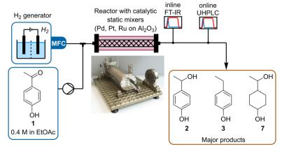
Fig. 1 Schematic representation of the setup used to study the hydrogenation of ketone 1, using different metal/Al<sub>2</sub>O<sub>3</sub> CSMs.
