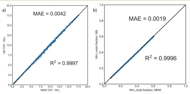
Fig. 2 Parity plots for DNN surrogate model for ammonia decomposition. a) Predicted turnover frequency (TOF) of NH<sub>3</sub> vs. the exact MKM. b) Exit mole fractions for NH<sub>3</sub> from 1200 PFR reactor simulations using the DNN-surrogate Python ODE solver model and the MKM (x-axis).
