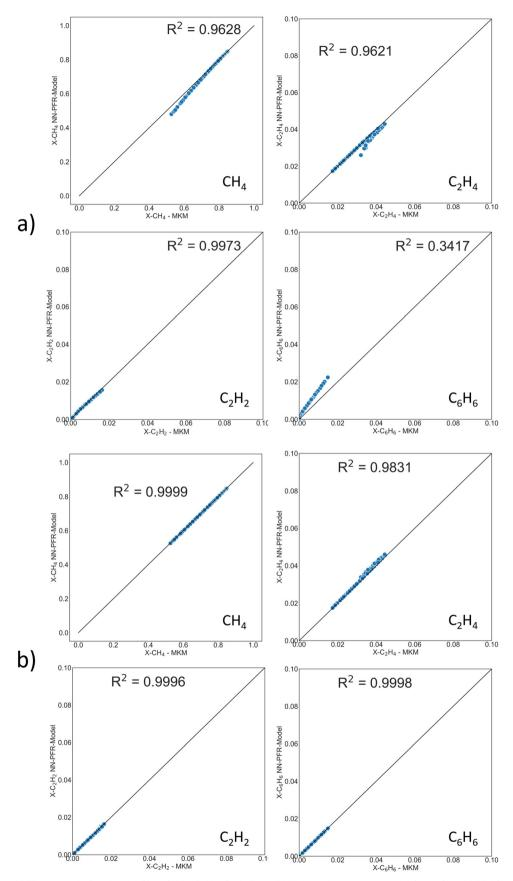
Fig. 5 Parity plots of PFR exit mole fraction of CH<sub>4</sub>,  $C_2H_4$ ,  $C_2H_2$ ,  $C_6H_6$  from DNN-based surrogate model (y-axis) and MKM (x-axis) for a) reaction set A and b) reaction set B. Trace reactions are considered for both reaction sets.
