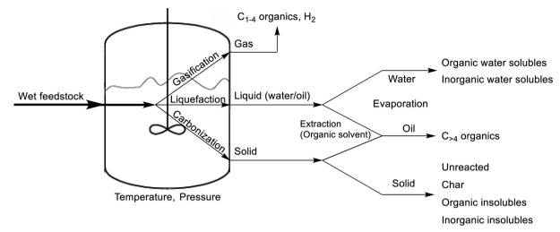
Scheme 1 HTL procedure with reactor and product distribution.
