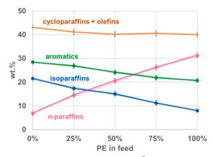
Fig. 8 Oil composition of HDPE: PP mixtures.8
