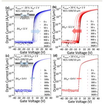
Fig. 5 Transfer characteristics under (a) PBS and (b) NBS for a-ITZO single-layer FET, and (c) PBS and (d) NBS for a-ITZO/a-IGZO FET. Stress conditions:  $V_{\text{stress}} = \pm 20 \text{ V}$  for 3600 s,  $V_{\text{DS}} = 1 \text{ V}$ . Enhanced PBS/NBS stability achieved through reduced electron trapping at the channel/gate dielectric interface or oxygen molecule adsorption at the back-channel
