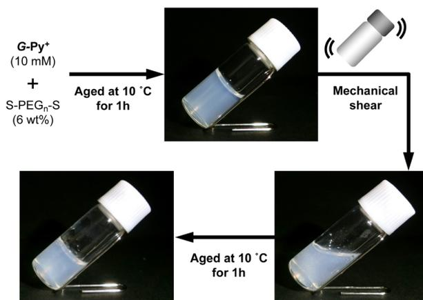
Fig. 6 Self-healing property of the hydrogel formed from an aqueous mixture of  $G\text{-Py}^+$  and  $S\text{-PEG}_{200}\text{-S}$  at 10 °C. The hydrogel was mechanically disrupted by vortexing.  $[G\text{-Py}^+] = 10 \text{ mM}$ ;  $[S\text{-PEG}_{200}\text{-S}] = 6 \text{ wt\%}$ .
