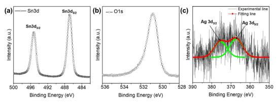
Fig. 4 High-resolution XPS of Ag TNPs/SnO<sub>2</sub>: (a) Sn 3d, (b) O 1s, and (c) Ag 3d.
