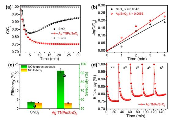
Fig. 5 (a and b) Photocatalytic NO removal ability and kinetic rates, (c) NO to  $NO_2$  and  $NO_3^-$  conversion efficiencies over  $SnO_2$  and Ag TNPs/ $SnO_2$ ; (d) stability test of photocatalytic NO removal over Ag TNPs/ $SnO_2$ .
