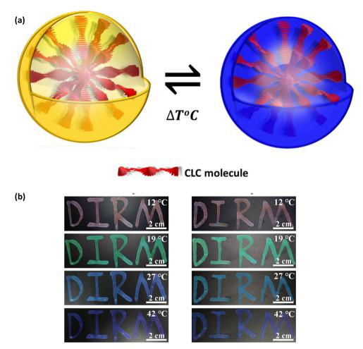
Fig. 6 (a) Principle of anticounterfeiting using temperature as stimuli (b) thermochromic coatings of cholesteric LC microcapsules with cellulose nanocrystals (CNC) and a melamine-formaldehyde (MF) resin hybrid shell with and without dye. Adapted from ref. 85 with permission. Copyright ©2022 American Chemical Society
