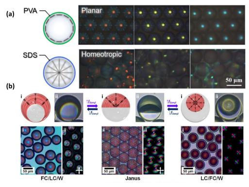
Fig. 4 (a) Cholesteric LC droplets exhibiting planar and homeotropic configuration. Adapted from ref. 74 with permission. Copyright © 2016 American Chemical Society. (b) Complex LC emulsions exhibiting dynamic reconfiguration in response to variations in surfactant content between F/LC/W double emulsions, Janus droplets, and LC/F/W double emulsions. Adapted with permission from ref. 75.
