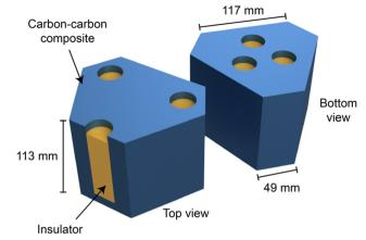
The schematic diagram of the six-sided polygon-shaped RHS is depicted, where the yellow and blue areas indicate the insulating container for the radioisotope and the carbon composite material, respectively. This figure is redrawn by the authors based on the original figure.8
