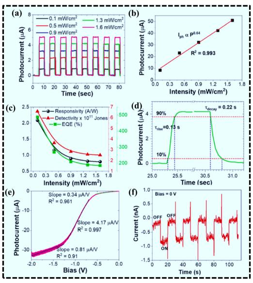
Fig. 11 (a) Time dependent photo response of the  $Ag-WS_2$  photodetector device at different illumination intensities, (b) photocurrent with respect to the illumination intensities, (c) responsivity, detectivity and EQE of the photodetector device, (d) rise and decay time constant, (e) photocurrent with respect to the applied bias potential and (f) time dependent photo response under an applied bias potential of 0 V. Reprinted with permission from ref. 141, Copyright of Elsevier 2021.
