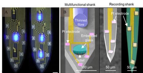
Fig. 7 Optical probes and injectable optoelectronics. (A) High-magnification images of the illuminated micro light-emitting diodes (scale bar: 15  $\mu\text{m}$ ). Reproduced with permission from ref. 74. (B) A multifunctional, implantable optoelectronic device. Reproduced with permission from ref. 75.
