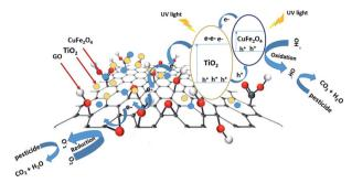
Proposed mechanism describing the process of charge separation in TiO<sub>2</sub>/GO/CuFe<sub>2</sub>O<sub>4</sub> through a direct Z-type scheme when exposed to UV light. Reprinted with permission from ref. 132 Copyright 2020, The Royal Society of Chemistry.
