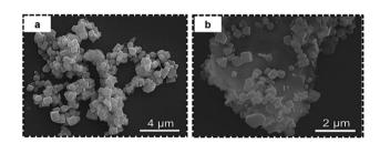
Fig. 26 SEM image of (a) Cs<sub>2</sub>AgBil<sub>6</sub> showing agglomerated particles and (b) GO/Cs2AgBil6 showing less agglomerated particles. Reprinted with permission from ref. 138 Copyright 2023, Elsevier.
