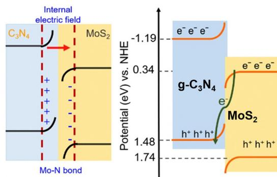
Fig. 13 Direct Z-scheme heterojunction illustration of GCN/MoS<sub>2</sub>. Reprinted with permission from ref. 84 Copyright 2023, the American Chemical Society.
