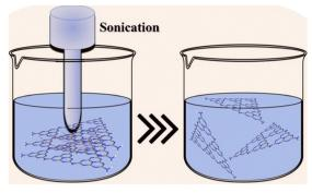
Fia. 4 Schematic illustration of the ultrasonic exfoliation method. Reprinted with permission from ref. 60 Copyright 2023, Elsevier.
