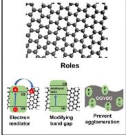
Fig. 1 Schematic illustration of the advantages of carbon nitride- and graphene-based materials for photocatalytic wastewater treatment. Graphitic carbon nitride as an active photocatalyst and its improvement strategies, with the role of graphene-based material in supporting the main photocatalyst.
