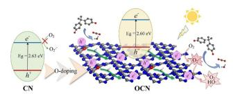
Fig. 11 Illustration of the photocatalytic reaction mechanism of OCN Reprinted with permission from ref. 78 Copyright 2022, Elsevier.
