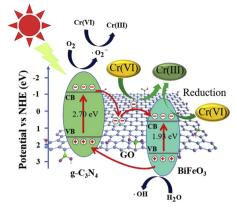
Fig. 21 Illustration of the potential process for the photoreduction of Cr(vi) over the CNGB-2 heterojunction when exposed to visible light. Reprinted with permission from ref. 125 Copyright 2019, Elsevier.
