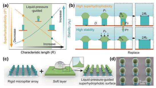
Fig. 11 Design of a bilayer-structural liquid-pressure-guided superhydrophobic surface (reproduced from ref. 149 with permission from [Wiley], copyright [2022]).
