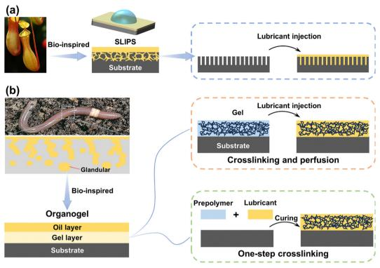
Schematic representation of the bio-inspired surfaces: (a) SLIPSs and (b) organogels and their preparation methods
