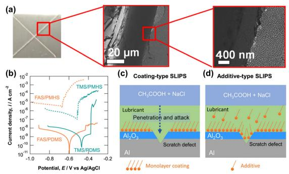
Fig. 19 Potentiodynamic polarization curves of the additive-type SLIPSs measured after immersion in 2 g dm<sup>-3</sup> acetic acid containing 10 g dm<sup>-3</sup> NaCl (pH 3) for one week and subsequent introduction of the scratch defects, and schematic illustrations of coating-type and additive-type SLIPSs with a scratch defect (reproduced from ref. 208 with permission from [American Chemical Society], copyright [2021]).
