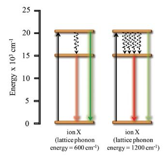
Fig. 3  $\,$  The effect of lattice phonon energy on the luminescence properties of an ion. Reprinted with permission from Wiley.<sup>48</sup>
