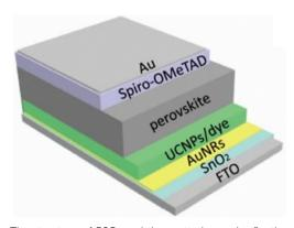
Fig. 16 The structure of PSCs and the scattering and reflecting mechanism diagram. Reprinted with permission from the American Chemical Society.  $^{74}$
