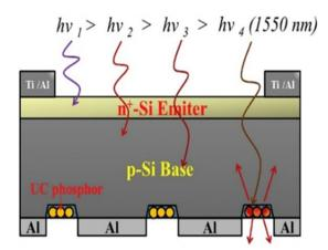
Fig. 20 A schematic diagram showing a silicon solar cell with  ${\rm SiO_2}$  coating containing YF<sub>3</sub>:Yb<sup>3+</sup>/Er<sup>3+</sup> phosphor particles within the backside matrix grooves for use in the upconversion of photons under excitation by a light source with a wavelength of 1550 nm. Reprinted with permission from Elsevier.<sup>77</sup>
