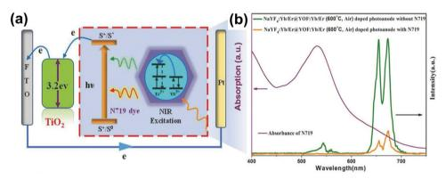
Fig. 10 (a) Energy diagram illustrating the NIR light-harvesting by the N719 dye through the UC process, the charge injection into  $TiO_2$  and the transport of photoelectrons to the electrode surface. (b) The absorption spectra of the N719 dye and the UC emission spectra of  $TiO_2$  photoanodes with NaYF<sub>4</sub>:Yb<sup>3+</sup>/Er<sup>3+</sup>@YOF:Yb<sup>3+</sup>/Er<sup>3+</sup> (600 °C, air) before and after immersion in N719 dye. Reprinted with permission from Wiley.<sup>88</sup>
