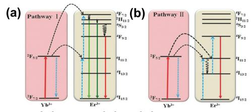
Fig. 9 The energy levels of the  $Yb^{3+}/Er^{3+}$ -codoped  $NaYF_4:Yb^{3+}/Er^{3+}$ @YOF: $Yb^{3+}/Er^{3+}$ , showing possible energy transfer upon 980 nm excitation. Reprinted with permission from Wiley. 88
