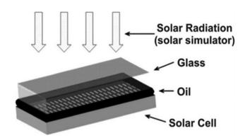
Fig. 18 A Si solar cell covered with glass and the matching oil. Reprinted with permission from Elsevier.95
