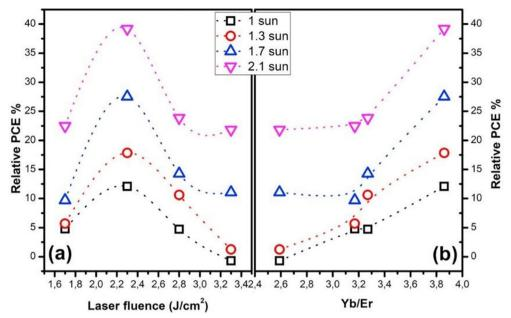
Fig. 21 The relative PCE dependence on the laser fluence (a), and (b) the Yb/Er elemental ratio measured at different solar simulator incident powers. Reprinted with permission from Elsevier.<sup>75</sup>
